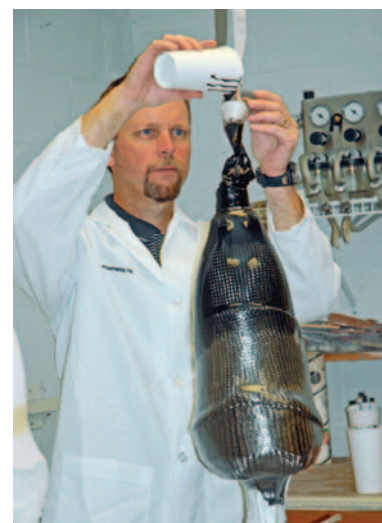
Adding catalyst-pigment mixture to activate socket lamination.
